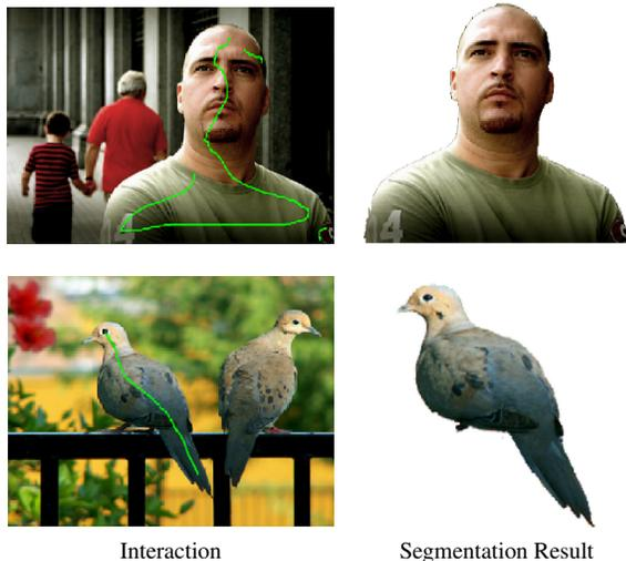
**Fig. 1:** User interactions and corresponding segmentation results
